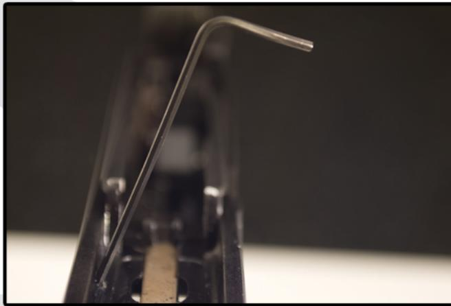
Remove trigger pin. The pin should only be removed out the left side of the frame. Attempting to remove the pin from the right side of the frame can damage the pistol and should never be done.
