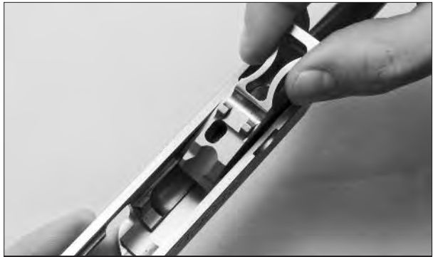
Figure 7. Installing Unlock Block
