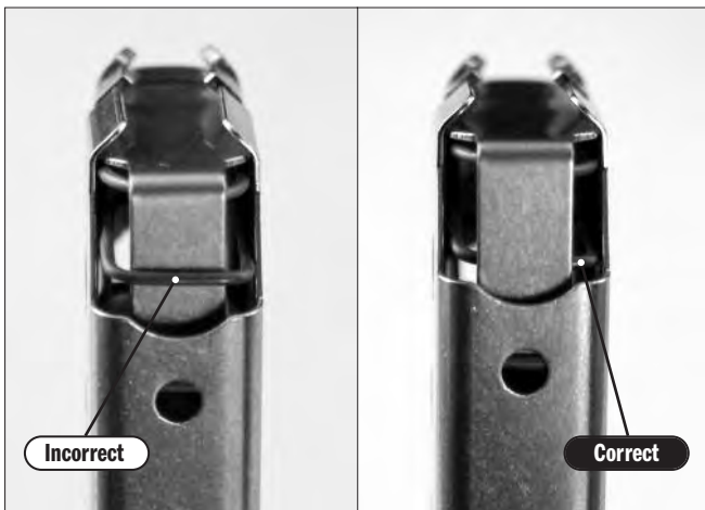
Figure 32. Proper magazine spring position under follower
