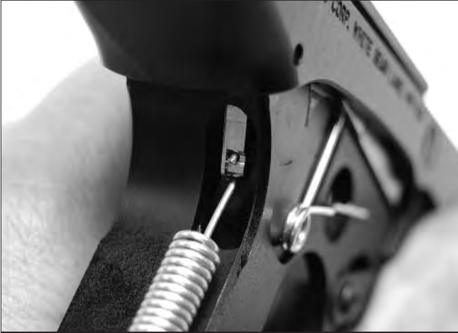
Figure 29. Correct Mainspring attachment
