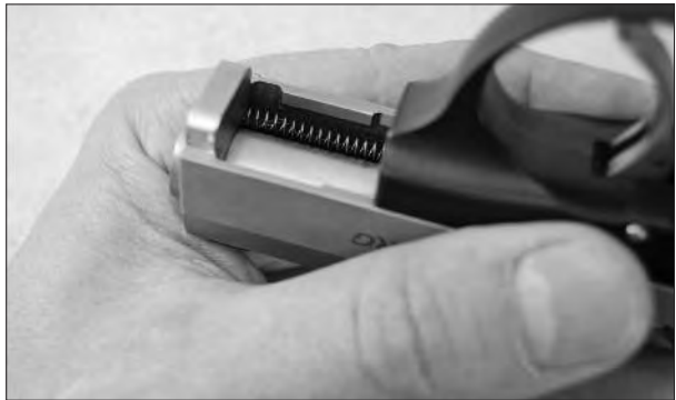
Figure 8. Recoil Spring Seated in Corner of Slide
