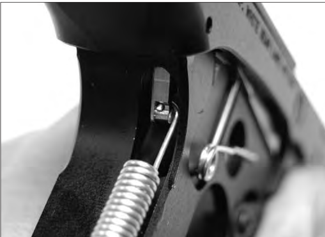
Figure 30. Incorrect mainspring attachment
