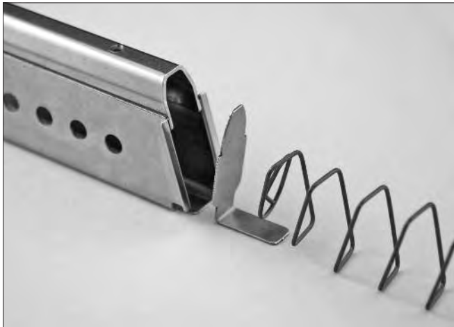
Figure 31. Proper insertion of magazine follower
