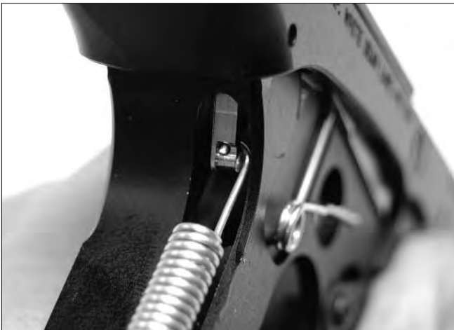
Figure 30. Incorrect mainspring attachment
