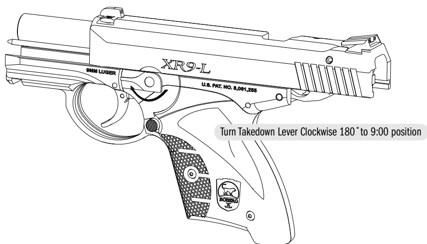
Figure 4. Field Strip—Takedown Lever at 9:00 Position
