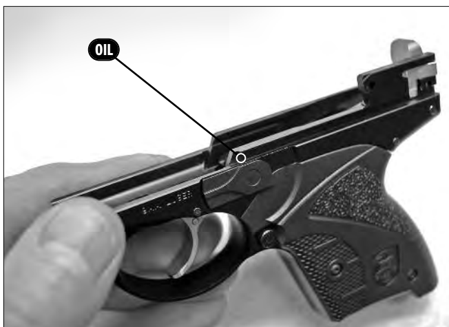
Figure 15. Left Slide Rail oiling point
