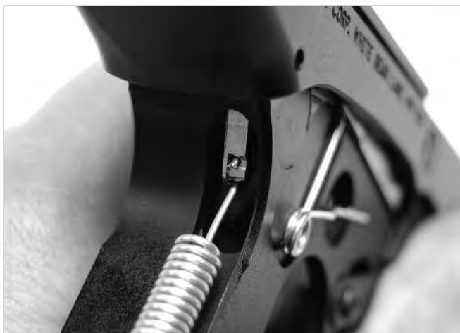
Figure 29. Correct Mainspring attachment
