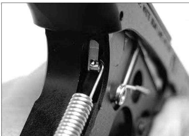
Figure 30. Incorrect mainspring attachment
