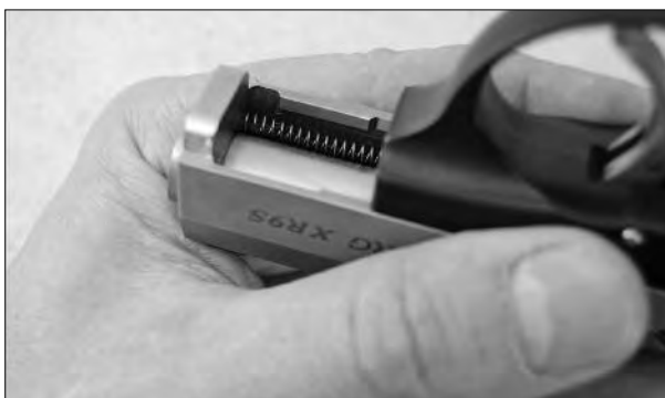
Figure 8. Recoil Spring Seated in Corner of Slide
