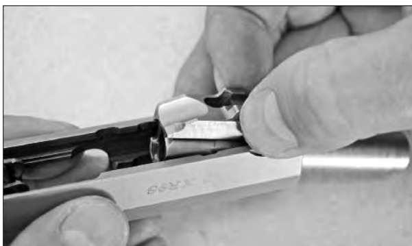
Figure 7. Installing Unlock Block
