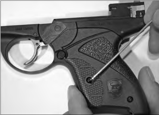
Figure 27. Remove Grip Screws
