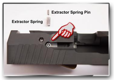
Place extractor spring and extractor spring pin in slide as shown.
