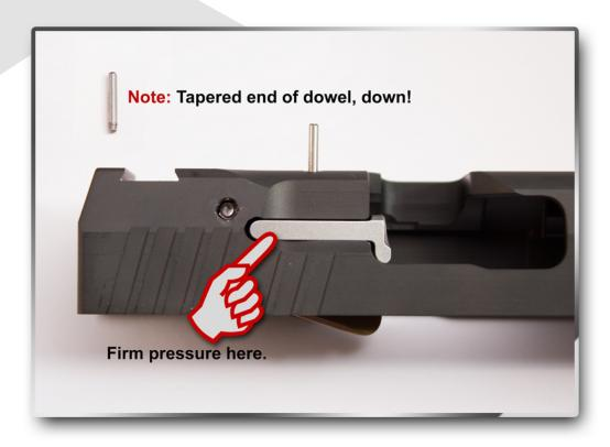
Place extractor in slot over spring. Place small amount of retaining compound on tapered end of dowel and insert into hole as shown. While applying firm pressure to area indicated, press pin into slide with a hard, non marring tool.
