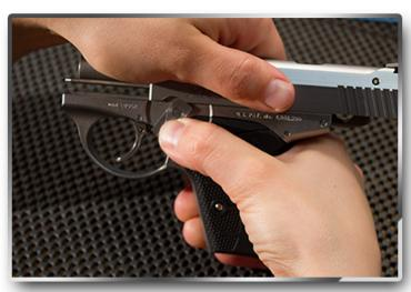
Remove slide, rotating slide release lever clockwise to the nine o-clock position.
