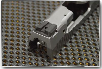
Apply loctite to the sight screw before installing and tightening.
