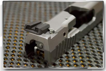
Place FP Safety Spring into the top of your slide as shown. You DO NOT NEED TO REMOVE SLIDE FROM FRAME TO REPLACE THE FIRING PIN SAFETY SPRING!
