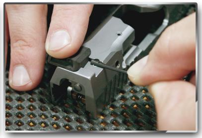
Depress the spring with an allen wrench as shown, making sure it is completely flush with the surface of the dovetail in your slide.
