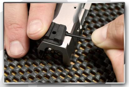
Slowly slide the rear sight into place, using the edge of the sight to push the allen wrench out of the way. The wrench will keep the spring from getting caught between the sight and the slide.
