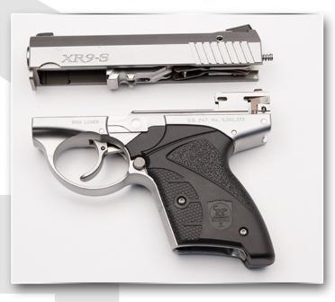
Remove slide, rotating slide release lever clockwise to the nine o-clock position.
