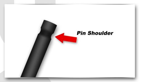
Reverse this process to reassemble the firearm. NOTE the 20 degree offset set screw that holds in the hammer pivot pin! Utilize a medium strength thread-lock on each set screw. Insert pivot pins through LEFT side of frame. Make sure "shoulder" of pivot pin is on the side that will interface with the set screw!
