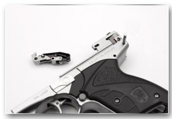
Partially remove hammer pivot pin. Allow pin to remain in frame far enough to retain the hammer as shown. This will allow the lift mechanism to be removed without removing the hammer. Remove lift mechanism.
