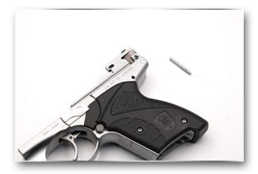
Remove lower link pivot pin from frame. Pin comes out of the left side of frame as shown. Removing the pin from the right side of the frame will damage the frame.
