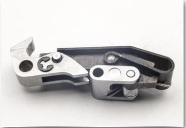
To install the "e-clip" on the flip link pin, lay the e-clip on the flip link as shown and use the blade of a flat head screwdriver or other similar tool to snap the clipinto the groove in the pin. Make sure e-clip is snapped into the groove and not above it.
