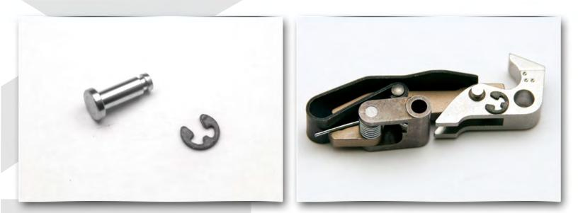
To install the "e-clip" on the flip link pin, lay the e-clip on the flip link as shown and use the blade of a flat head screwdriver or other similar tool to snap the clipinto the groove in the pin. Make sure e-clip is snapped into the groove and not above it. While the e-clip will remain on the pin if not seated into the groove, it will work its way off during firing!
