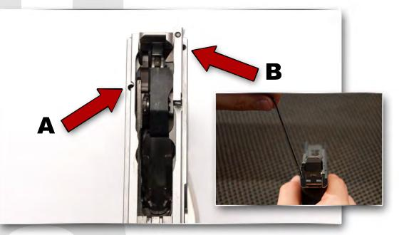
Remove the set screws at points indicated. Use a .050 inch allen wrench. Set screw "B" is at a 20 degree offset, make sure to properly seat the wrench.
