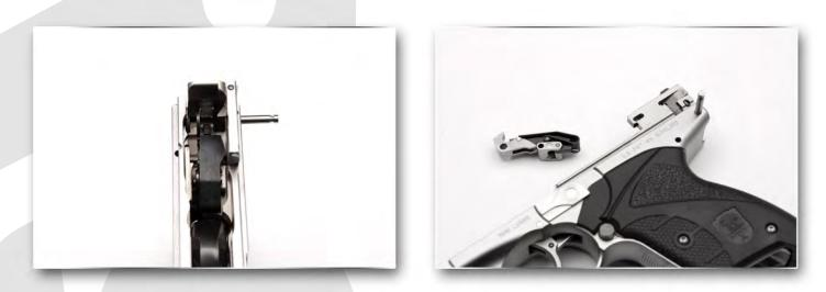
Partially remove hammer pivot pin. Allow pin to remain in frame far enough to retain the hammer as shown. This will allow the lift mechanism to be removed without removing the hammer. Remove lift mechanism.
