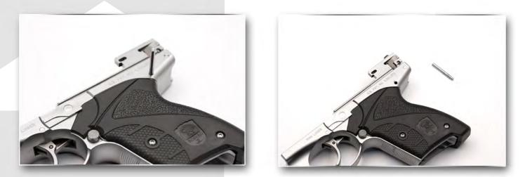
Remove lower link pivot pin from frame. Pin comes out of the left side of frame as shown. Removing the pin from the right side of the frame will damage the frame.
