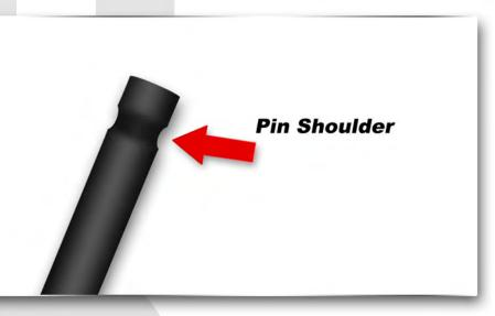
Reverse this process to reassemble the firearm. NOTE the 20 degree offset set screw that holds in the hammer pivot pin! Utilize a medium strength thread-lock on each set screw. Insert pivot pins through LEFT side of frame. Make sure "shoulder" of pivot pin is on the side that will interface with the set screw!
