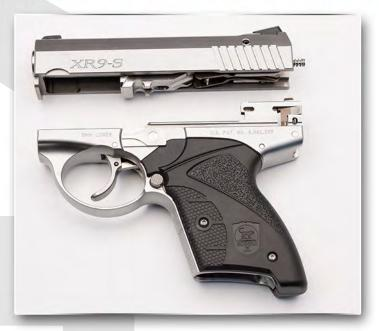
Remove slide, rotating slide release lever clockwise to the nine o-clock position.
