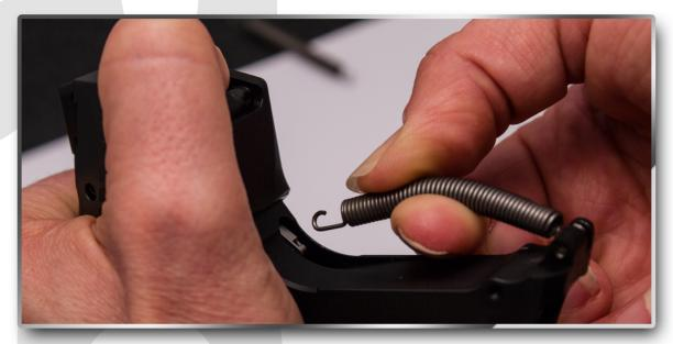
While applying pressure to hammer, attach "long" end of mainspring to the end of anchor link that protrudes from under the back-strap of the pistol.
