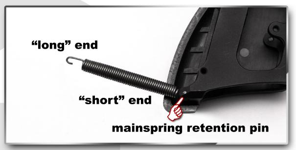
Attach "short" end of mainspring to mainspring retention pin with the "open" side of hook facing towards the back of pistol as shown.
