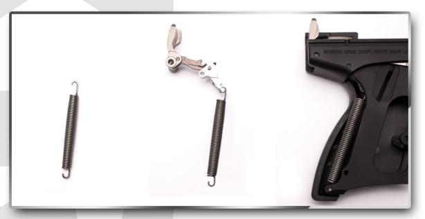
Mainspring. Hammer assembly and frame shown for position reference.
