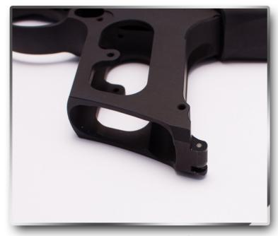
Retaining pin should be flush with frame. Evidence of thread-lock should be visible on both ends of pin!
