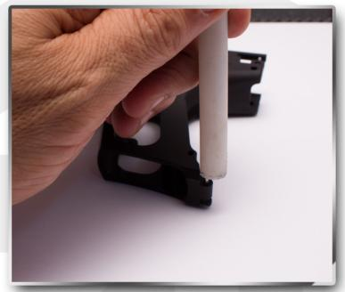
Using a plastic rod and mallet, force pin TAPERED SIDE DOWN, into hole in frame.
