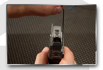
Note the lift link pivot pin set screw (B.) goes into the frame at a 90 degree angle!
