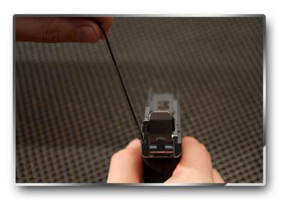
Note the hammer pivot pin set screw (C.) goes into the frame at a 20 degree offset!
