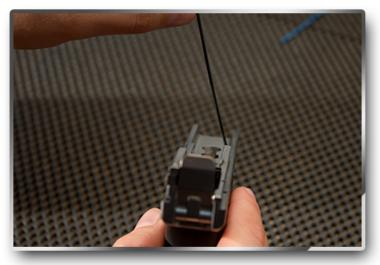
Note the trigger pivot pin set screw (A.) goes into the frame at a 20 degree offset!
