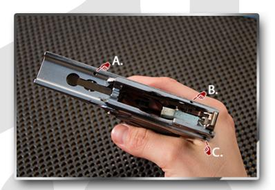
Note the three set screw positions for the trigger, lift link and hammer pivot pins.
