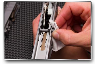
Use a fold of cloth or glove to protect fingers and rotate lever back from the 2 o-clock position to the 10 o-clock position while removing lever.
