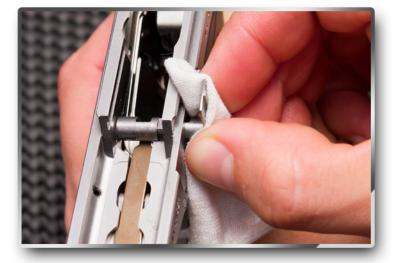
Protect fingers with a fold of cloth or glove and rotate lever back and forth while pressing lever into frame.
