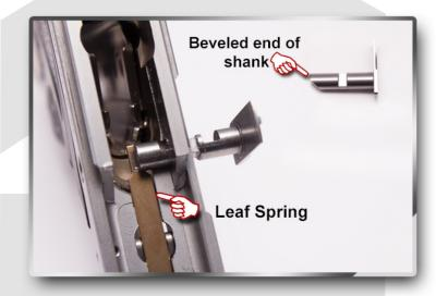
Insert lever pointing to 12 o-clock position until beveled end of shank sits on top of leaf spring.
