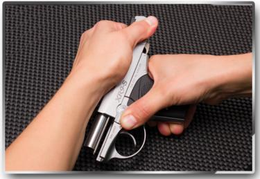
Remove slide, rotating takedown lever clockwise to the nine o-clock position.
